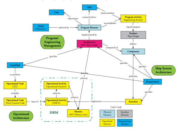
Fig. 6. Ship Design System Architecture (adapted from Vitech, 2010)
