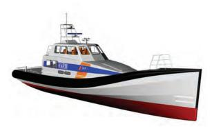
From an extensive series of experiments carried out with a model of this new design and a model of the existing boat in the towing tank, it has been demonstrated that a considerable improvement in the head seas conditions has been achieved with the new concept, without any loss of performance under following and stern quartering conditions.
