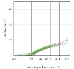
Fig. 7b. The distribution of the vertical accelerations at the bow for the Conventional Catamaran at 25 knots in irregular waves with significant wave height Hs of 1.5 m.
