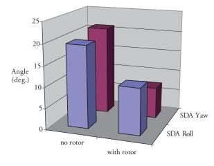
Fig. 15. Maximum Roll and Yaw angles with and without the Bow Rotor at 22 knots in a seaway from an angle of incidence of 315 degrees with a significant wave height of 3.5 meters
