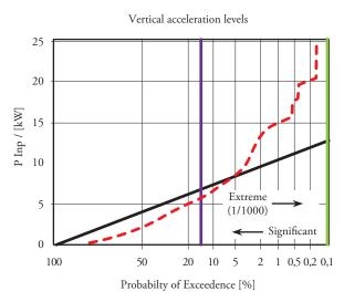
The wish to avoid the high peaks in the acceleration signal for improved operability in a seaway means that a distribution according to the black (straight) line is very much to be preferred above the distribution following the red line. This holds true even though the significant value corresponding with the black distribution line is higher than that of the red line.
