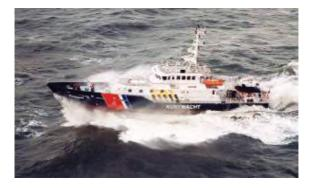
performance. These have to be operated from low to moderate sea states in particular for application as service vessels for the offshore wind mill farms at the North Sea. Typical length of these vessels is in the 20-meter range and typical speeds are up to 25 knots in calm water. In addition to the usual requirements for low levels of vertical accelerations
