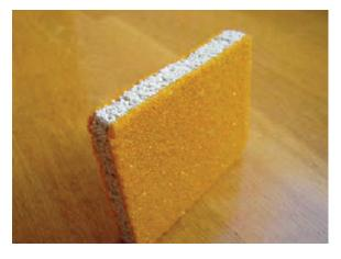
Fig.7b. Building material from recycled composites. Gypsum blocks
