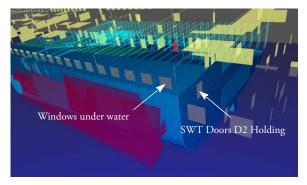
Fig. 14. Time-Domain Simulation of the Flooding Process (various openings)
