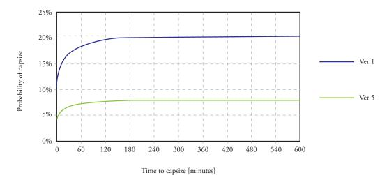
Fig. 15. Cumulative probability distribution for time to capsize within a given time for two ship layouts shown in Figs. 6 and 7
