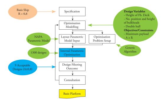
Fig. 5. Platform Optimisation Process - Concept Designs
