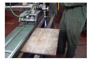
Fig. 5. Test coupon for Naval Steel of the type ASTM A131 Gr A of Steel made in 2008 and steel made in 1972. Prior to welding.
