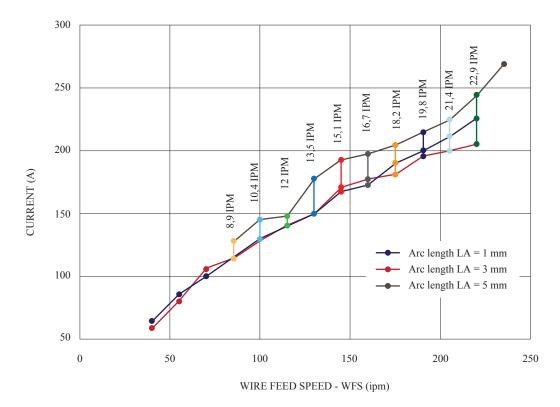
Fig. 12. Graphic with the Current relationship VS WFS
