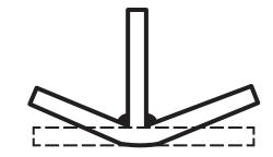
Fig. 2. Angular and buckling deflections due to the stiffeners welding of a panel-type structure (ANSI/AWS D 3.5:93R, 1993)
