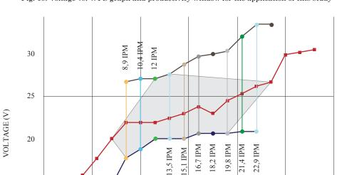
Fig. 10. Voltage vs. WFS graph and productivity window for the application of this study
