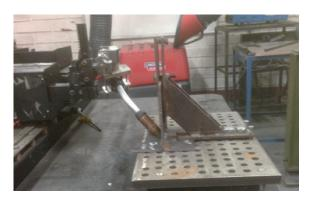
(C) Pistol and coupon arrangement in 2f
