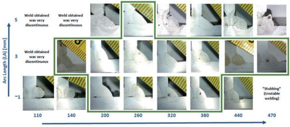
Fig. 9. Photo-ultrasounds with the shape of the welding beads according to the welding parameters
