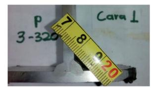
Fig. 8. Macro-photography of welding applied with WFS= 320 ipm and LA = 3 mm
