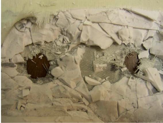
a) High content alumina and mullite ceramic (AM2). View of the rear face of the plate after being impacted by a projectile (NATO Ball FMJ 7.62x51mm). Backing material was removed
