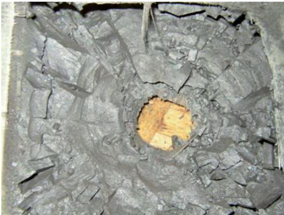
b) Biomorphic ceramic (RBS) impacted by 7.62x63mm AP-M2 projectile
